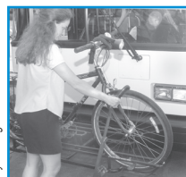
3. Secure the bike by clamping the bar over the tire
